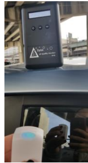
Figure 29. Above: Dylos sensor; Below: Wynd sensor
